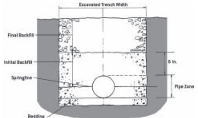
4. The trench should be completely filled. The backfill should be placed and spread in fairly uniform layers to prevent any unfilled spaces or voids. Large rocks, stones, frozen clods, or other large debris should be removed. Heavy tampers or rolling equipment should only be used to consolidate only the final backfill.
